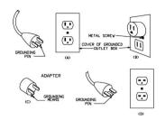
**WARNING:** This heater has a voltage rating of 120 volts. The cord has a plug as shown in A. An adapter as shown in C is available for connecting three-blade grounding- type plugs to two-slot receptacles. The grounding lug extending from the adapter must be connected to a permanent ground such as a properly grounded outlet box. The adapter should not be used if a three-slot grounded receptacle is available.
